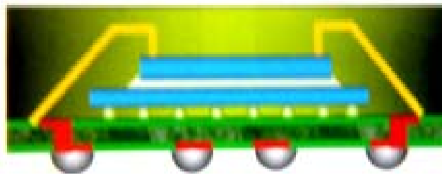
Figure 33: Hybrid package combining wire bond and flip chip for 3D SiP
